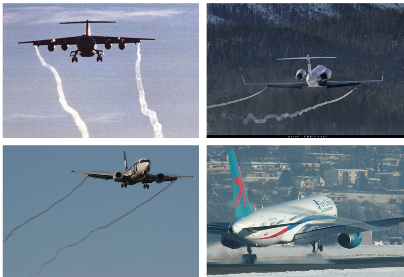
Fig. 1 Photographs showing condensation in flap-edge vortices. The source of the lower two figures is www.airliners.net . All photographs are reproduced with permission.
